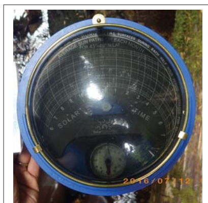
Figure 6. Example Solar Pathfinder Image Used to Estimate Effective Shade.
