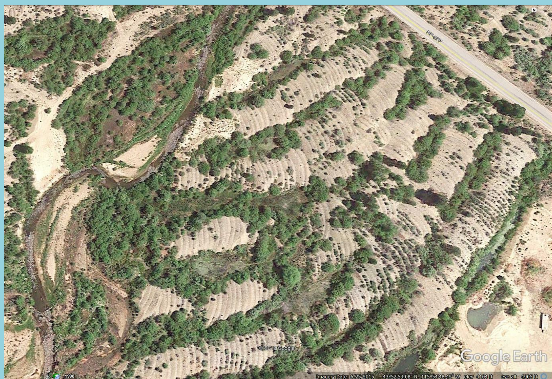
Dredge tailings, Grimes Creek
