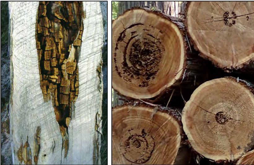
Figure 48. Decay caused by cedar brown pocket rot shown in lengthwise- (left) and cross-sections (right).
