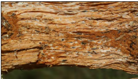
Figure 16. Decay from Heterobasidion (annosus) root disease showing laminated decay with black flecks.
