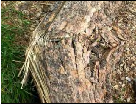
Figure 70. Tension and compression branch failure. On the right side of this branch, fibers are folded from compression; at left, tension caused fibers to pull apart and splinter.
