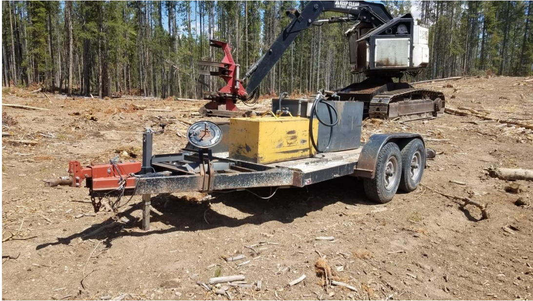
Figure 15: Uncontained fuel storage tank
