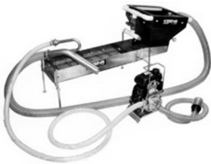
Figure 5. Power sluice/suction dredge combination
