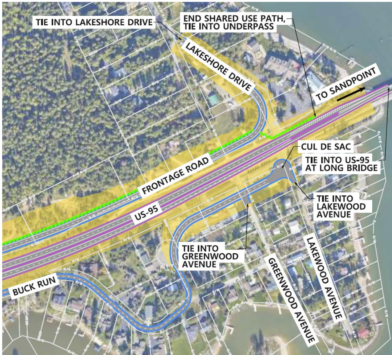
Figure 3. US-95 Proposed Action - Access Controlled Highway and Frontage Roads
