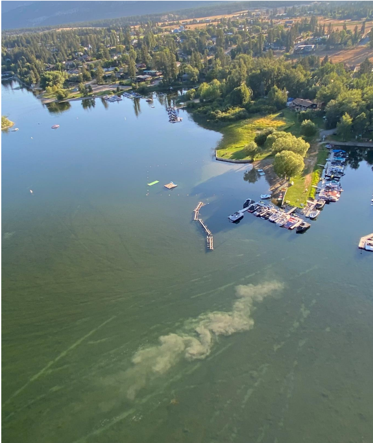
Figure 7: Aerial image of sediment plume from a wake-surf boat operated in shallow water. Note the tracks through the sediments from other boat passage, all emanating from the marina.
