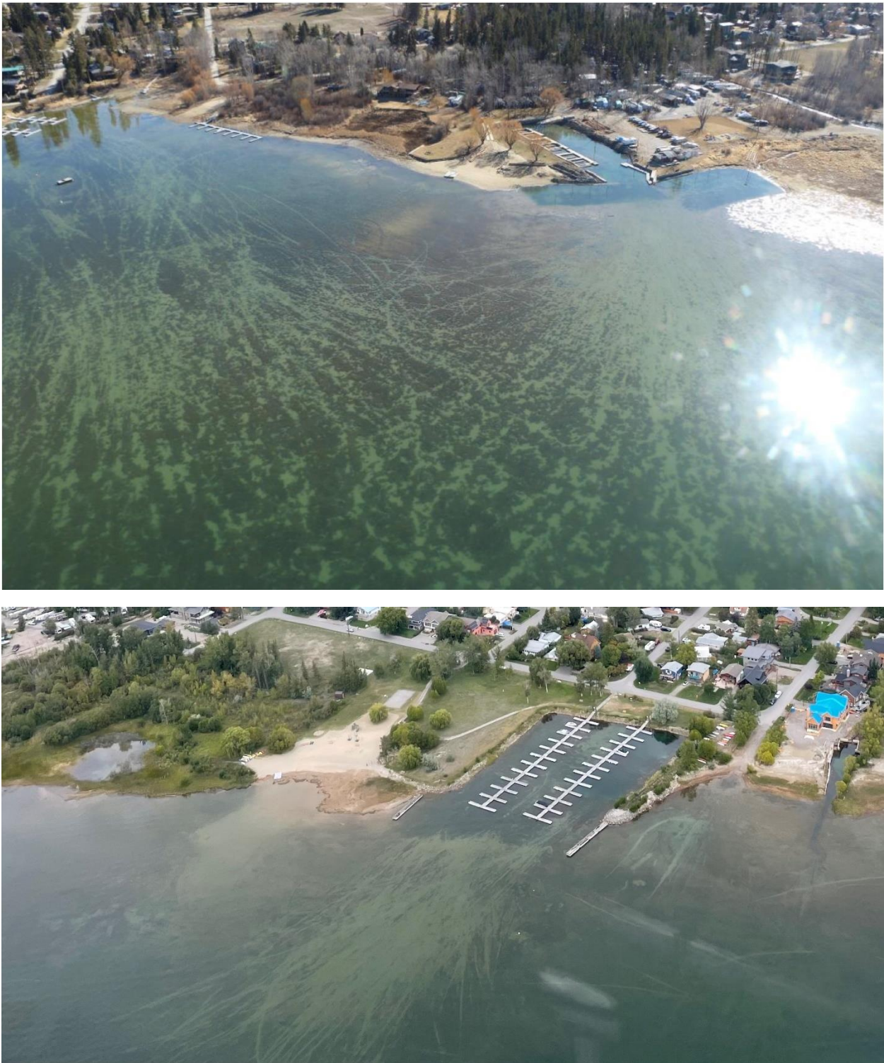
Figure 15: Sediment scouring along boat travel routes from marinas, Lake Windermere 2024 (Photo from LWA)
