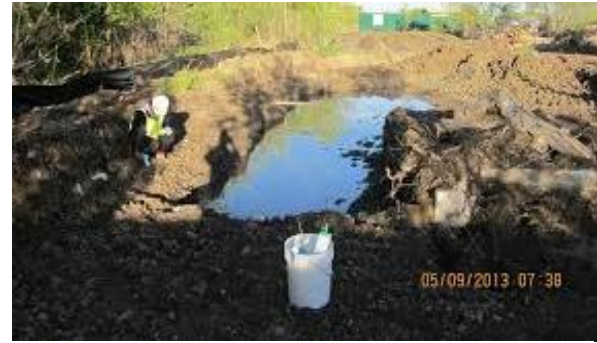
Confirmation soil sampling at the Murray Laundry Superfund site in Salt Lake County, Utah. The EPA removed contaminants at this site to address threats to public health and the environment. (EPA photo)
